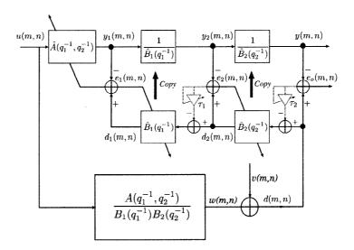
Figure 1. Equation error formulation for separable denominator 2-D IIR filters.
