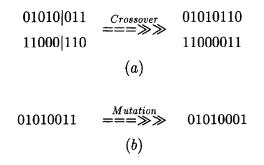
Fig. 1. (a) Crossover operation. (b) Mutation operation: the preultimate bit to the right is mutated from a 1 to a 0.
