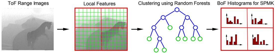
**Figure 2:** Local features for range images are computed on a grid without using interest point detectors. All local features are clustered with a Random Forest and used to compute Bag-of-Features (BoF) histograms for each cell. Only one level of the pyramid is shown in this figure.
