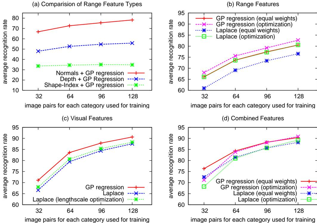
**Figure 4:** Evaluation of (a) different types of range features; (b) GP methods with multiple range features; (c) GP methods with colour features; (d) and combined features from the CCD camera and the ToF camera. 32 image pairs corresponds to one object instance or type.
