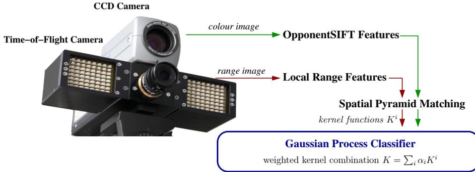
**Figure 1:** An overview of the proposed approach: colour and range images are captured using a CCD camera and a Time-of-Flight camera (PMD Vision Technologies 19k); Local features are extracted from the data of both sensors and “kernelized” using Spatial Pyramid Matching, yielding different kernel functions.
