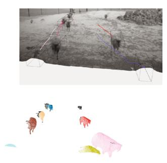
**Fig. 8.** 3D multiobject tracking using scene-flow (left). Instance clustering based on 2D mask projections (right).
