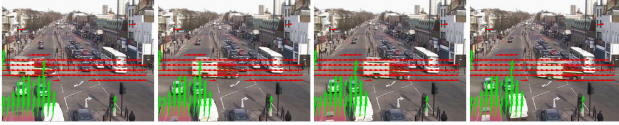
Figure 7. Detected abnormality in clip 4 of the Junction data-set, where a fire-engine interrupts traffic flow. (Some flow vectors have been removed to improve visibility.)
