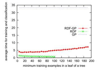
Fig. 3. Average computation time for Gaussian Processes, Random Forests and RDF-GP (measured in seconds).
