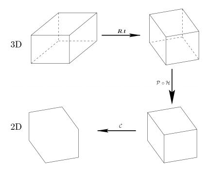
Figure 1: 3D bounding volumes for 2D contour prediction: The mappings  $\mathcal{P}$ ,  $\mathcal{H}$ , and  $\mathcal{C}$  are formally described in the text. By estimating the position of the bounding volume we can calculate the 2D contour in the image plane which is needed to initialize the active contour.
