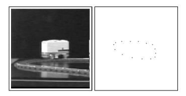
Figure 11: Correct result: experiment 1. Left the image, right the active contour.
