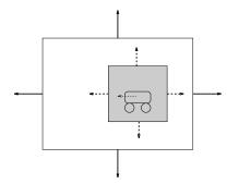
Figure 7: Two methods are used for changing the view of the scene: dashed lines indicate changing the parameters of the grabbing device; solid lines indicate the motion of the robot using a proportional controller. The large light rectangle is the field of view of the camera, the small gray rectangle is the area digitized on the board.
