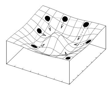
Figure 1: Principle of active contours: A snake with 7 elements extracts the contour of a circle by moving into the minimum of the negative edge strength of the circle.
