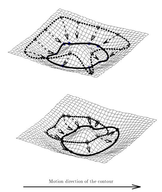
Figure 4: Tracking principle using active contour models (compare Figure 1). Top: The initial snake (dotted line) and the result of energy minimization (solid line). Bottom: Extraction of the contour in the next image. Result of the previous image (dotted line) converges to the contour of the circle (solid line), if the displacement of the object in the image plane is less than a maximum displacement given by the smoothing of the energy and the object's size.
