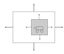
Figure 4: Two methods used for changing the view on the scene: dashed lines by changing the parameters of the grabbing device; solid lines by the motion of the robot. Only the grey area is digitized on the board.
