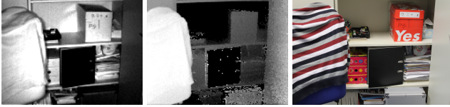
Figure 2. Intensity (left) and depth image (middle) recorded by a ToF camera. Right: Same scene recorded by a CCD camera.
